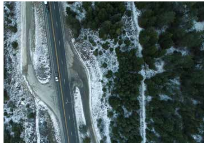
US-95 and Granite Loop Road/Old House Road Intersection prior to construction. High accident location located on hill with passing lane and low sight distance.
