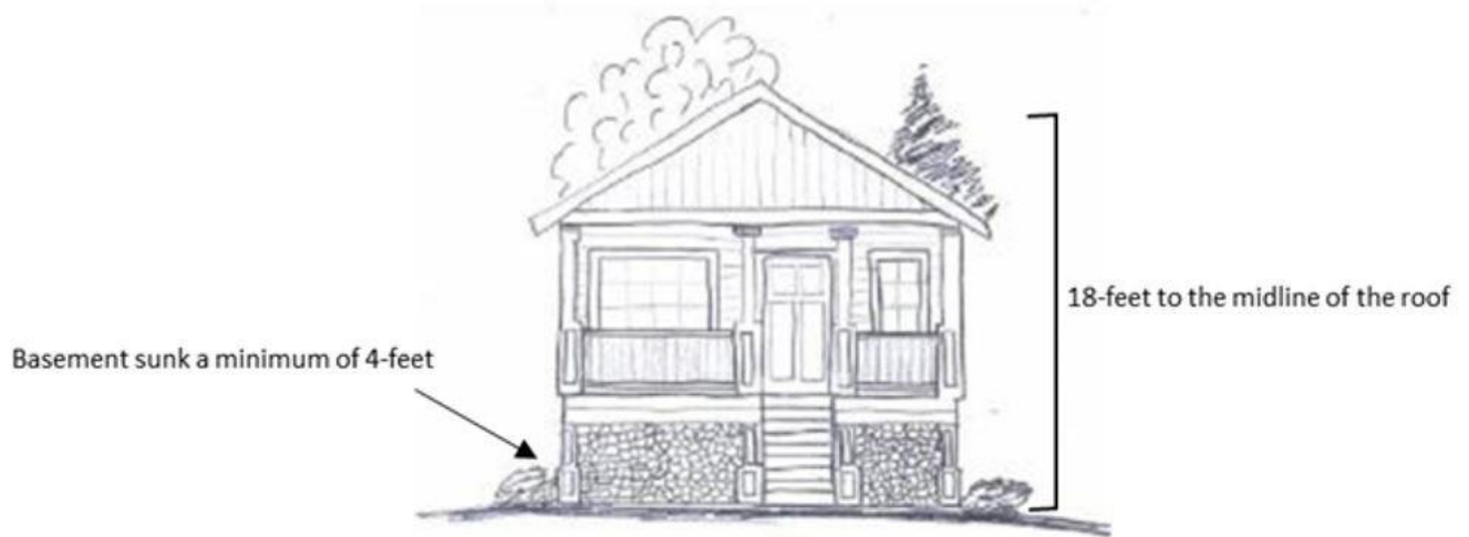
Figure 6.3: Example of second story within a basement
